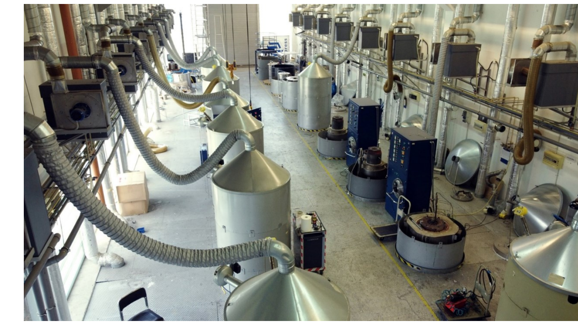
Hall of ammonothermal autoclaves.
