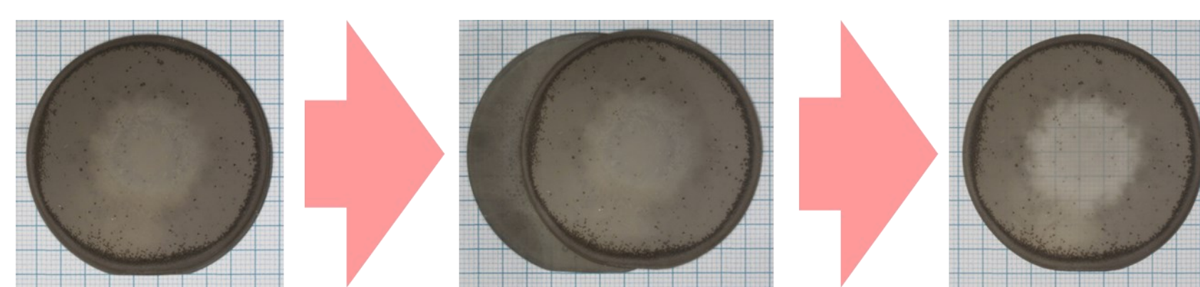
From the left a) GaN grown on MOVPE GaN/sapphire/Ti mask, b) self lift-off, c) 2-inch 1-mm-thick free-standing HVPE-GaN.
